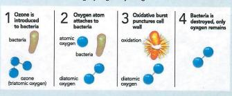
When ozone-saturated bubbles are mixed with water in your tank the weaker oxygen molecule in the ozone separates and binds itself to any organic molecules existing in the water. The organic molecule is then oxidised and destroyed.
